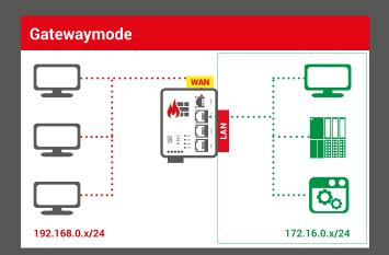
In **Gatewaymode**, WAN and LAN interfaces will each get a different IP address, thus segmenting the original network. With this setup, functions such as NAT and Forwarding can be used to route data traffic to secondary networks. Meanwhile the packet filter manages data exchange between WAN and LAN.
