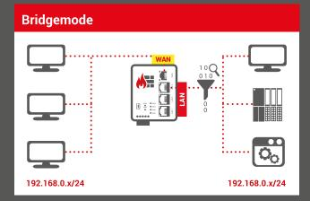
In **Bridgemode**, mbNETFIX fits easily into existing networks without changing any network range and protects data exchange between its interfaces, filtering packets between WAN and LAN. It integrates transparently, so no IP address allocation is necessary.
